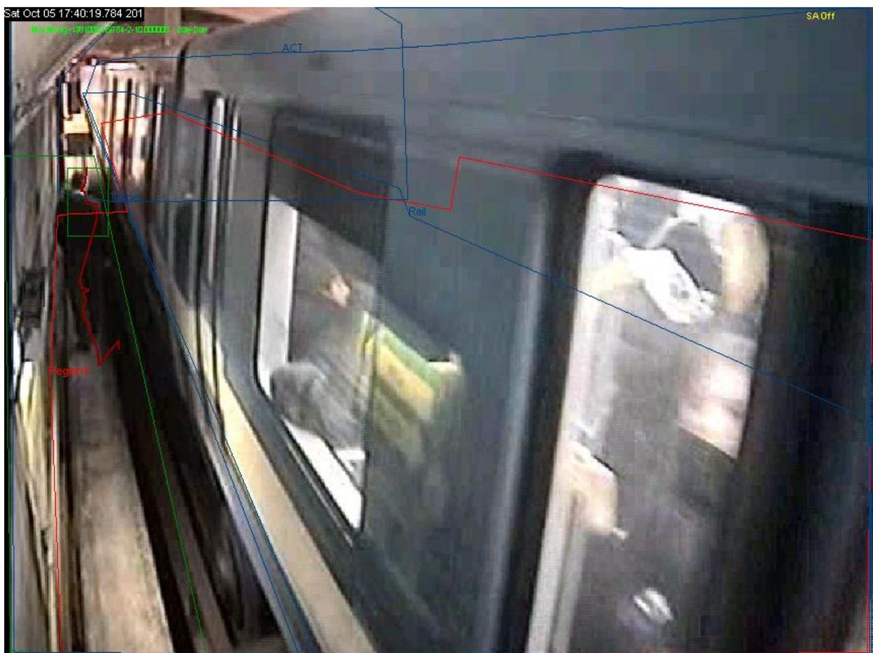
**Figure 3 -- Intruder detected by SmartCatch on a catwalk next to a moving train in the Montreal Metro**
