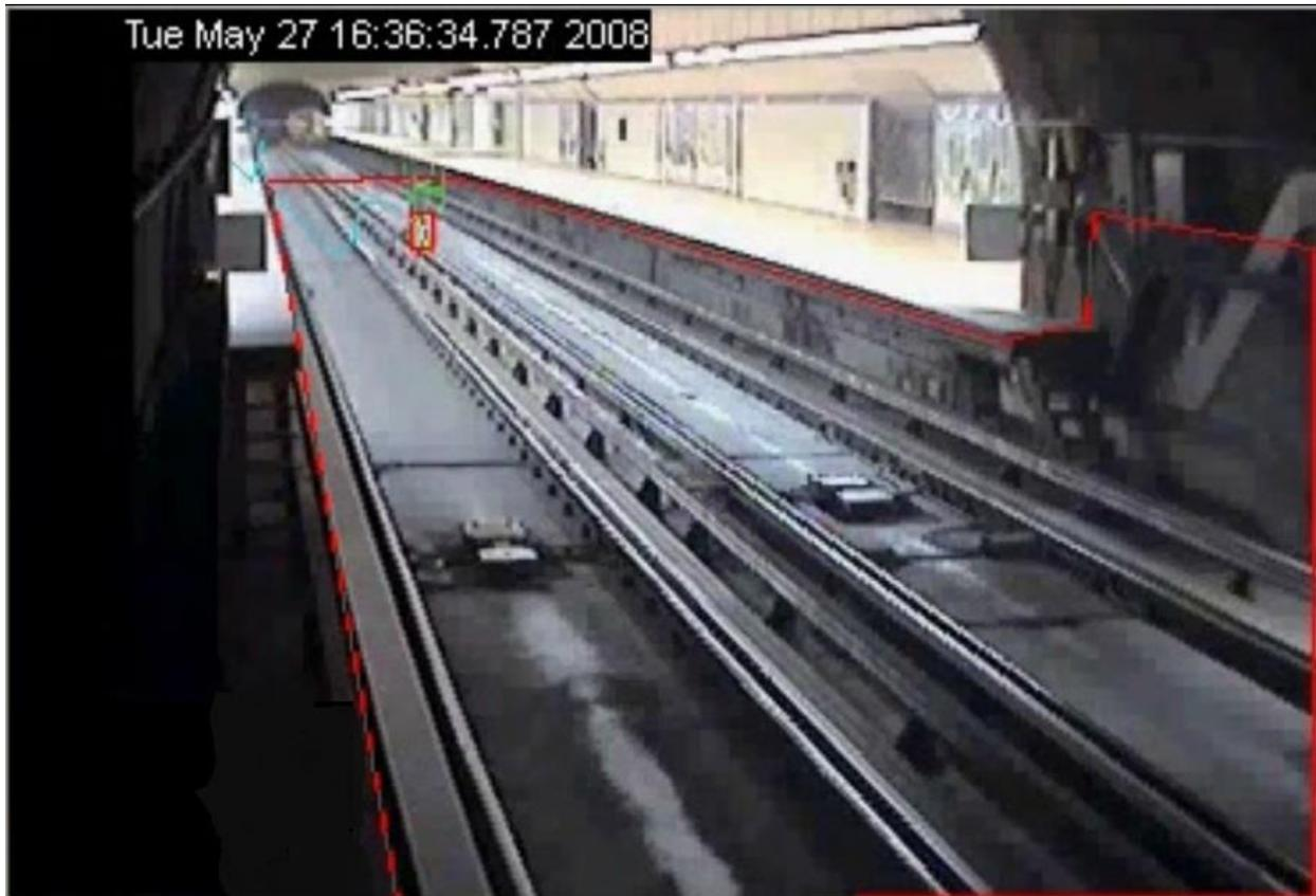
**Figure 2 -- Small human figure detected by SmartCatch on the tracks in the Montreal Metro**
